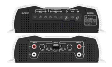
HPF/ LPF: 90Hz (-12dB/8°) fixed Input impedance: 10K ohms Dimensions (WxHxL): 6.81"x2.05"x8.94" Weight: 3.15 lb
