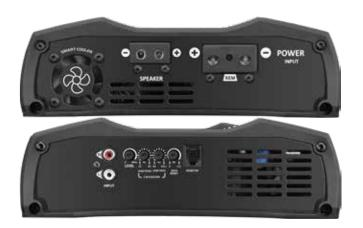
HPF: 10Hz to 80Hz (-12dB/8<sup>a</sup>) variable LPF: 80Hz to FULL (-12dB/8<sup>a</sup>) variable Input impedance: 10K ohms Dimensions (WxHxL): 8.98"x2.76"x21.65"
